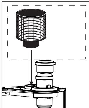
Push the air filter into the air intake on top of the boiler. See figure 14b.
