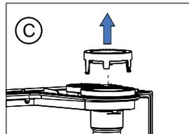
C. Push out the 5" cover from the vent connection (=air intake)
