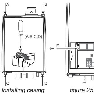
To commission the boiler the casing has to be removed.
