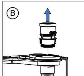
B. Pull the 3" connection out of the boiler
